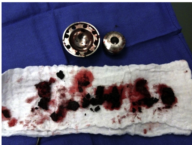
Fig. 1. Tissue is shown from a pseudotumor debrided during revision of the acetabular component in a 42-year-old female patient with failure secondary to metal complication at 6.5 years postoperatively.
